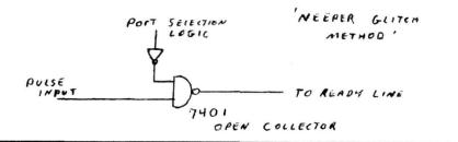
When the port device is selected, the input strobe goes low causing the ready line to go low stopping the processor. The processor goes into a wait state. Only when a signal is applied to the pulse input does the processor run again.
