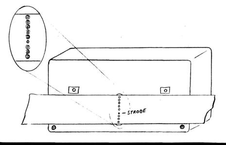
When you are certain good allignment is possible, peel the backing from the mask and <u>gently</u> (without stretching) apply from the center out, and recheck for allignment.
