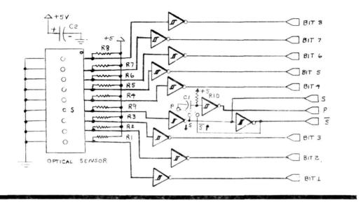
The heart of the PTR-II is a precision 9-element silicon photo readhead. The elements of this optical sensor have been specially matched to greatly increase its reliability and reduce the circuitry.
