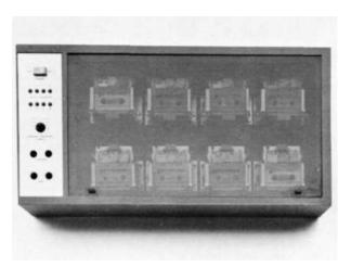
write operations. The VIATAPE bank control panel indicates which VIATAPE cartridge is being referenced by the current operation. Tape and operational characteristics are identical to those of the VIATAPE cartridge recorder.
